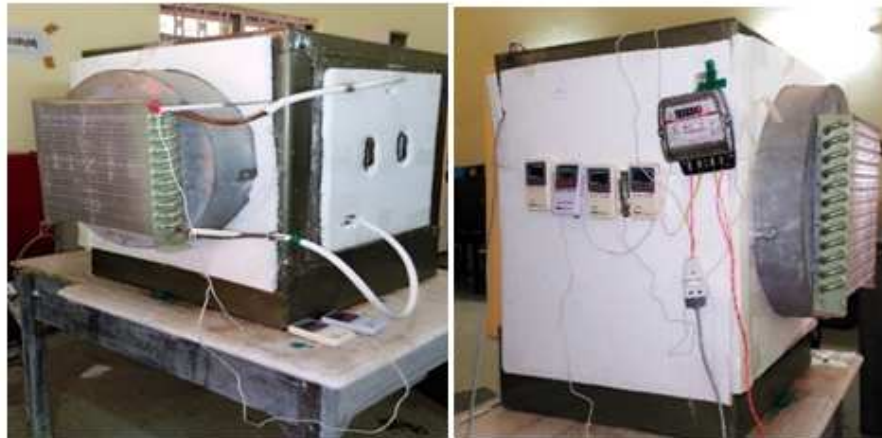
Arrangement of Instrument to Measure Temperature at Different Points
